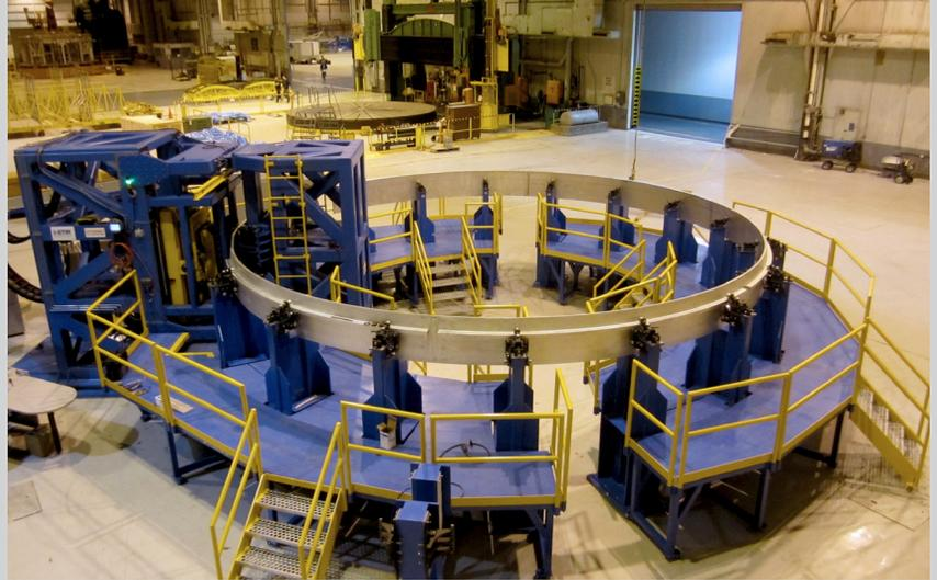
The Segmented Ring Tool will use a friction stir weld process to produce segmented support rings for the SLS core stage. *(Image: Futuramic)*
