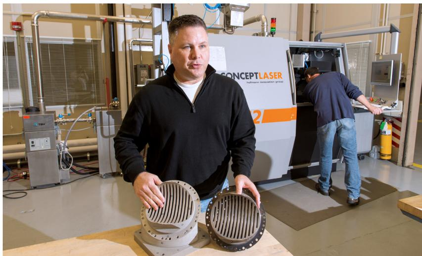
Andy Hardin, SLS Subsystem manager for liquid engines, compares a rocket engine part created using traditional manufacturing and welding, on right, with one made one using Selective Laser Melting, or SLM, on left. The new z-baffle for the RS-25 engine was created by fusing metal dust with a high-power laser using the machine in the background. (Image: NASA/MSFC)
