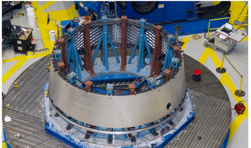
An adapter that will connect the Orion spacecraft to its rocket for EFT-1 is under construction at NASA's Marshall Space Flight Center in Huntsville, Ala. The same design will be used for the flight test of the full-size Space Launch System rocket in 2017. (Image: NASA/MSFC)
