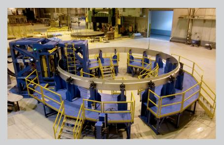
The Segmented Ring Tool will use a friction stir weld process to produce segmented support rings for the SLS core stage. *(Image: Futuramic)*
