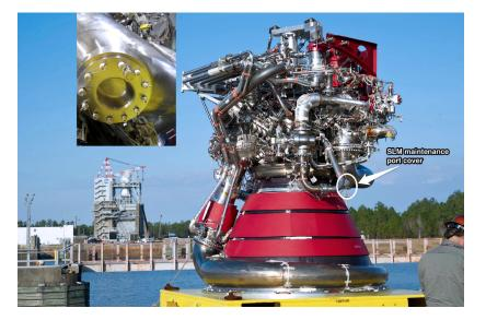
The J-2X engine before installation at the Stennis Space Center. The engine's new turbo pump exhaust port cover (detailed inset) was recently built by Pratt & Whitney Rocketdyne of Canoga Park, Calif., using a pioneering manufacturing process called Selective Laser Melting. *(Image: NASA/SSC)*
