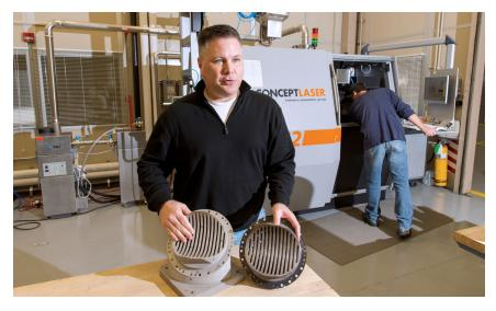
Andy Hardin, SLS Subsystem manager for liquid engines, compares a rocket engine part created using traditional manufacturing and welding, on right, with one made one using Selective Laser Melting, or SLM, on left. The new z-baffle for the RS-25 engine was created by fusing metal dust with a high-power laser using the machine in the background. *(Image: NASA/MSFC)*
