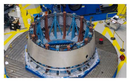
An adapter that will connect the Orion spacecraft to its rocket for EFT-1 is under construction at NASA's Marshall Space Flight Center in Huntsville, Ala. The same design will be used for the flight test of the full-size Space Launch System rocket in 2017. *(Image: NASA/MSFC)*
